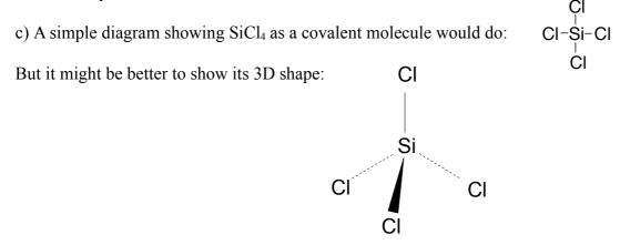
Silicon(IV) chloride is a liquid at room temperature because the forces between one SiCl<sub>4</sub> molecule and its neighbours are only van der Waals dispersion forces. These don't take anything like as much energy to break as ionic bonds.
