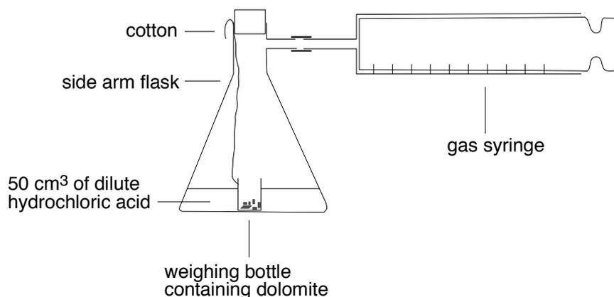
Collection of gas over water into an inverted measuring cylinder is an acceptable alternative. Pieces of dolomite in weighing bottle so that reaction can be started with no loss of gas. Description should include shaking the flask to upset the weighing bottle, followed by constant shaking, and recording the volume of gas in syringe at 30 second intervals.
